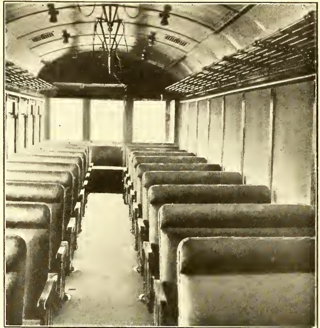
JAMESTOWN CARS—INTERIOR VIEW OF PASSENGER COMPARTMENT, SHOWING FULLY GLAZED MOTORMAN'S COMPARTMENT IN RIGHT-HAND CORNER
